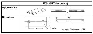
Note: The shape of the adhesive tape shown above is for securing the F03-16PE.
