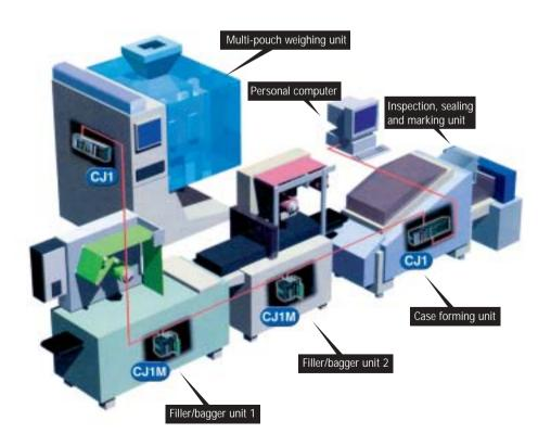
The CJ1 controllers let you scale control capability to match the needs of each machine unit for flexible reconfiguration. Manage production using data transferred via network from the PLCs on each machine to a personal computer.
