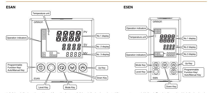
\* A 2-level display when shipped from the factory. A 3-level display is activated if parameters are initialized. For details on the third display level, refer to the *User's Manual, Basic Type* (Cat. No. H156).
