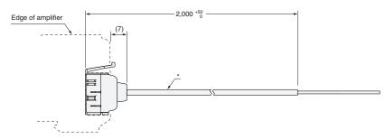
$^{*} \ E3X-CN12; \textbf{2.6 dia.} \ cable \ / \ \textbf{1 conductor} \ / \ Standard \ length: 2 \ m \ (Conductor \ cross \ section: 0.2 \ mm^{2} \ (AWG24), \ Insulator \ diameter: 1.1 \ mm)$
