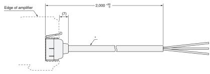
\* E3X-CN11: 4 dia, cable / 3 conductors / Standard length: 2 m (Conductor cross section: 0.2 mm2 (AWG24), Insulator diameter: 1.1 mm)
