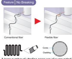
A large number of ultrafine cores are all surrounded by cladding. As a result, the fiber is flexible and can be bent without significantly reducing the light intensity. This helps solve problems, such as fiber being broken by getting caught on other objects.
