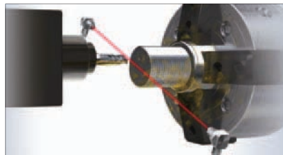
Detection of low-reflective workpieces such as black rubber
