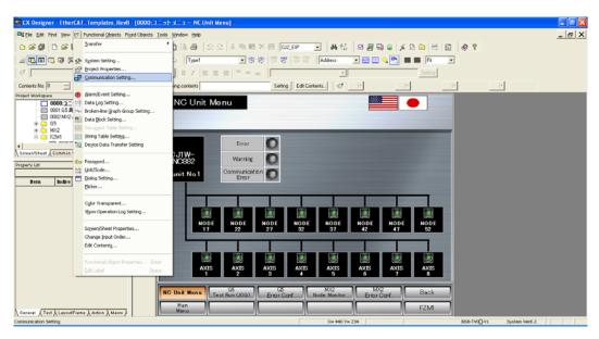
2. Right-click a communication channel and select to "Add..." a new Host, then adjust communication parameters as necessary and select OK.
