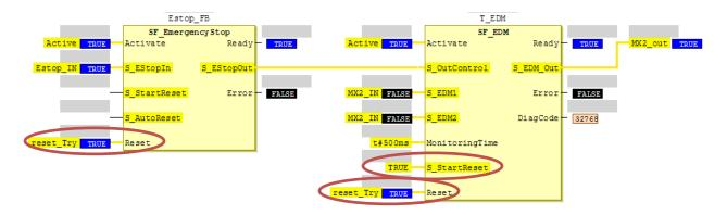
Use reset pushbutton (variable used in example: reset\_Try) input for all safety devices and EDM function blocks.
