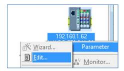
b. Modify the assembly sizes as shown. After modifying the sizes, edit the Tag sizes for the PLC / MAC, modify the Connection to reflect the new sizes, and download to the PLC / MAC.
