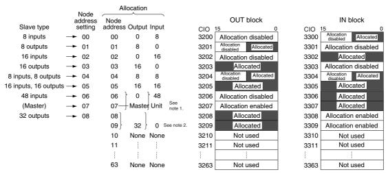
Note 1 The Master Unit does not require any word allocation and so it can use any available address.
