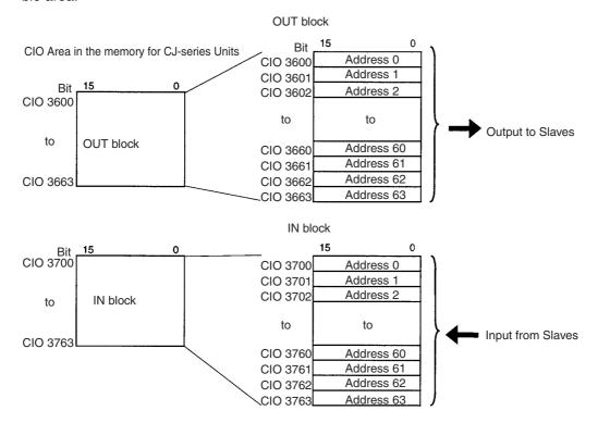
The Slave allocation order is fixed in the output (OUT) and IN blocks that start from address 0. Each address is allocated at least one byte (rightmost).
