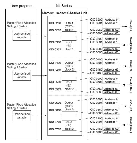
Specify using master fixed allocation setting switches 1-3.
