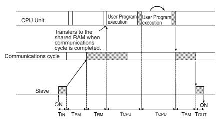
T<sub>IN</sub>: The Input Slave's ON (OFF) delay T<sub>OUT</sub>: The Output Slave's ON (OFF) delay T<sub>RM</sub>: Network's communications cycle time
