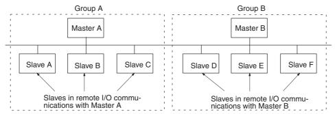
Although in the above diagram the Slaves are separated into two groups for convenience, the actual physical positions in the Network are irrelevant.
