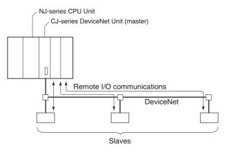
Note A CJ-series DeviceNet Unit can function as either a master or slave in remote I/O communications and it can even function as both a master and a slave at the same time. Change \* Sw1MstrEnblCmd (Master Enable Switch) to TRUE to set the CJ-series DeviceNet Unit to function as a master. Once master communications are enabled, the Unit will continue to perform master communications regardless of whether the power is turned OFF and back ON again.
