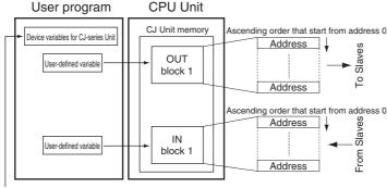
Specify the area, first word, and allocation size to allocate output/input block 1.
