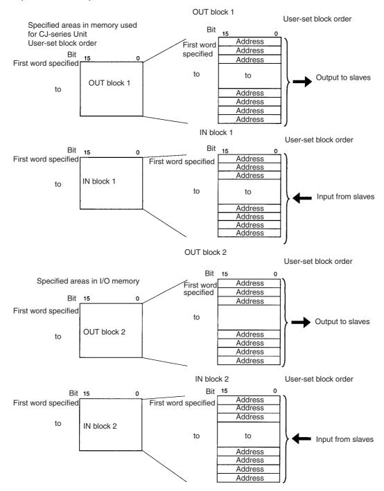
You can set the block allocation order, block allocation areas, and order of node addresses in each block. Each address is allocated at least one byte (rightmost or leftmost byte).
