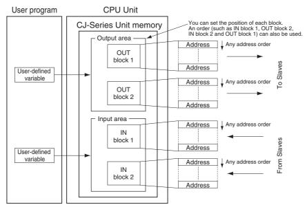
You can use any order for block allocations and for slave allocations within each block. Each address is allocated at least one byte (rightmost).
