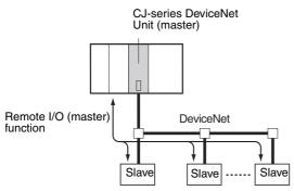
Note Refer to Section 4 Remote I/O Master Communications for details on remote I/O communica-
