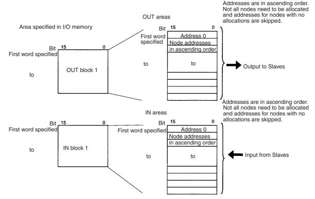
You can set the block allocation order and block allocation areas. Node addresses in each block are allocated words in ascending order from 0 to 63. Node addresses that are not allocated are skipped (not allocated words). Each address is allocated at least one word (rightmost byte, 1 word, or multiple words).
