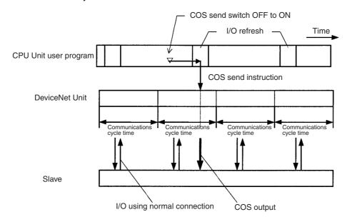
You can change multiple bits to TRUE simultaneously and you can send output data to multiple node addresses simultaneously.
