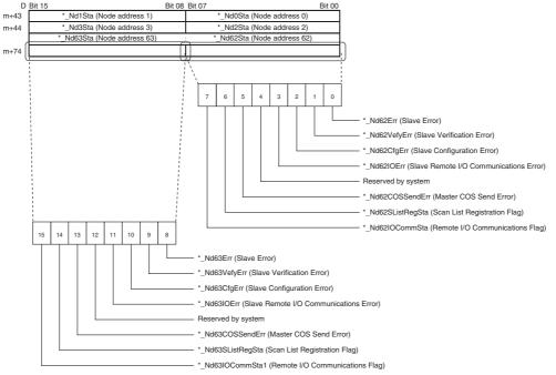
The device variables for CJ-series Units that correspond to bits 0 to 7 or 8 to 15 of each word are as follows:
