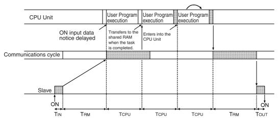
T<sub>IN</sub>: The Input Slave's ON (OFF) delay
