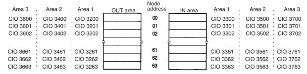
Note You can include more than one Master Unit in a single CPU Unit with fixed allocations, as shown below (3 Units max.).
