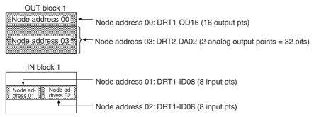
• Each address is allocated at least one byte (rightmost or leftmost byte).
