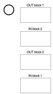
b) Node addresses do not have to correspond between an output block and input block.
