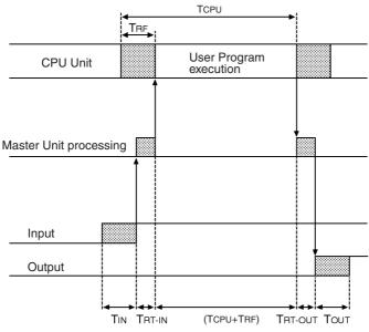
T<sub>IN</sub>: The Input Slave's ON (OFF) delay T<sub>OUT</sub>: The Output Slave's ON (OFF) delay
