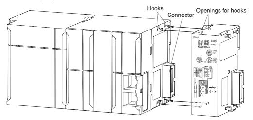
**2** Move the yellow sliders on the top and bottom of the Unit until they click into position, to lock.
