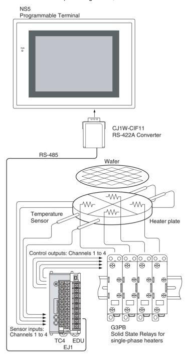
A single Temperature Controller can handle the 4-zone control if a 4-channel Basic Unit (EJ1□-TC4) is used. Up to 16 Basic Units can be connected to one EJ1C-EDU End Unit to expand to a maximum of 64 channels.
