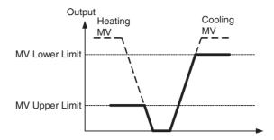
Output Mode Selection = Heating/cooling control
