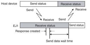
The setting of the Send Wait Time parameter can be shortened to reduce the communications time at the host device as long as there are no problems.
