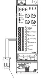
Set the baud rate to 57.6 kbps (default value) using key operations. For details, refer to the *G3PW Operation Manual*.
