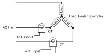
V Connection: Refer to the following diagram for CT installation positions.
