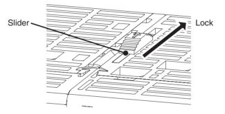
3. Attach the cover seal to the connector on the Unit on the left end of the EJ1.
