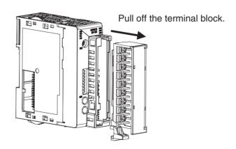
**Note** Screw and screw-less terminal blocks cannot be exchanged. Use the type of terminal block supplied with the TC Unit.
