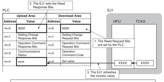
When the Read Request Bits are set (step 1), steps 2 and 3 performed automatically.
