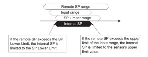
The remote SP's range will not be changed automatically, even if the input type or SP Limiter is changed.
