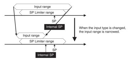
**Note** The SP is not changed, but the internal SP used for control is limited by the upper limit of the input range.
