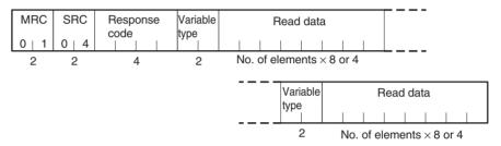
The read data is read together with the variable type, in the order specified in the command.
