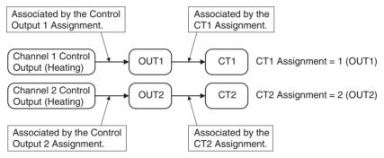
Example 2 Three-phase heater burnout detection is performed on channel 1's control output (heating).
