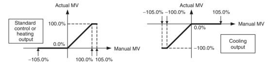
Use an event input or operation command to switch between auto mode (standard control) and manual mode. When using an event input to switch modes, set the Event Input Assignment parameter to Auto (0)/Manual (1). After the event input is set, it will operate as follows:
