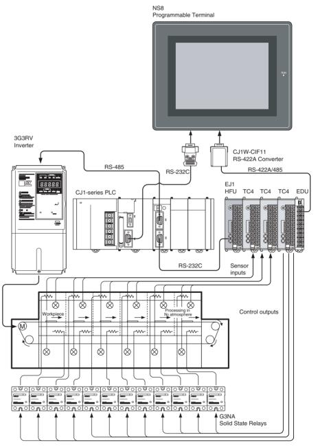
If an EJ1□-HFU is used, a ladder program does not have to be created to exchange data such as temperature readings and alarm status with the PLC.
