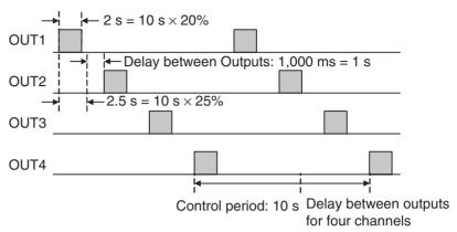
**Note** The Delay between Outputs parameter can be set to offset the ON time for each output. The delay between outputs will, however, create an OFF period between outputs, making it appear that the control period has increased. The actual power is  $2/(10 + 4) \times 100 = 14.3\%$ .
