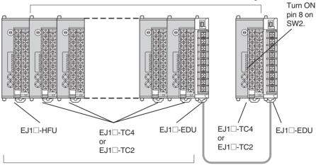
Up to 16 Units can be connected side by side.
