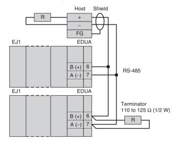
The RS-485 connection can be either 1: 1 or 1: N. RS-232C connections can only be 1: 1. A maximum of 64 Units (including the host) can be connected in 1: N systems. The maximum total cable length is 500 m. Use AWG28 (cross-sectional area: 0.081 mm²) to AWG16 (cross-sectional area: 1.309 mm²) shielded twisted-pair cable.
