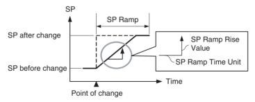
The rate of change during SP ramp operation is specified by the SP Ramp Rise Value, SP Ramp Fall Value, and SP Ramp Time Unit parameters. The SP ramp function will operate when the SP Ramp Rise Value or SP Ramp Fall Value is not set to 0 (disabled).
