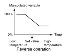
For example, when the process value (PV) is lower than the set point (SP) in a heating control system, the manipulated variable increases according to the difference between the PV and SP. Accordingly, this is "reverse operation" in a heating control system and "direct operation" in a cooling control system, which performs the opposite operation.
