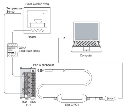
• The CX-Thermo Support Software can be used to set EJ1 parameters from the personal computer.
