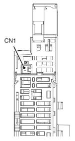
Connect the G3ZA Connecting Cable to the CN1 connector on the bottom of the TC Unit.
