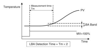
(3) Set the LBA Detection Time parameter to two times the measured time.
