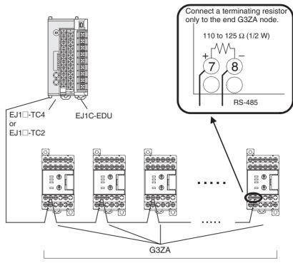
Up to 8 G3ZA Power Controllers can be connected to one TC Unit.
