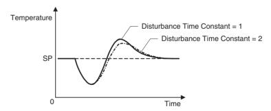
**Note** The waveform shown in the diagram above will vary depending on the control object's characteristics and the PID constant settings.
