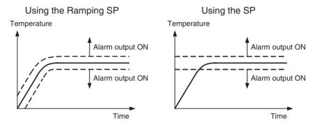
**Note** The alarm type is set to 1 (Upper and lower limit).
