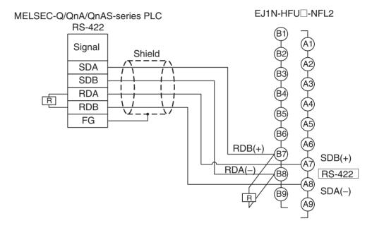
Recommended Example of RS-485 Wiring We recommend the following wiring for RS-485 communications to maintain transmission quality.
