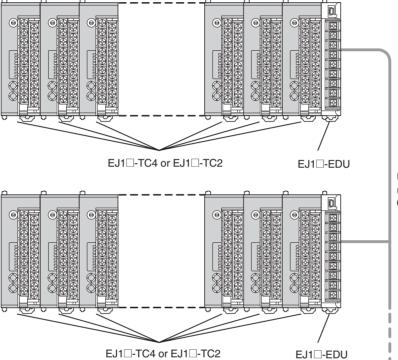
Up to 64 Basic Units can be connected using distributed placement (4 channels  $\times$  64 Units = 256 channels).
