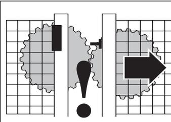
Check the machine is isolated and stopped whenever the interlocked guard door is open.
