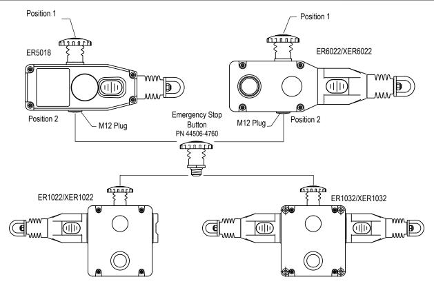
The ER-Series and XER-Series Rope Pull E-Stop Switches are designed to allow the Emergency Stop Button to be re-positioned, replaced, or added in the field. The ER5018, ER6022 and XER6022 have two positions in which the Emergency Stop Button may be mounted. Only one Emergency Stop Button may be installed per switch. The ER/XER1022 and ER/XER1032 have only one position to install the Emergency Stop Button.
