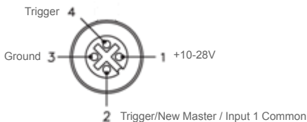
QX-1 Trigger Connector 4-pin Socket
