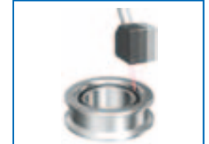
Measuring Depth of O-Ring Insertion
