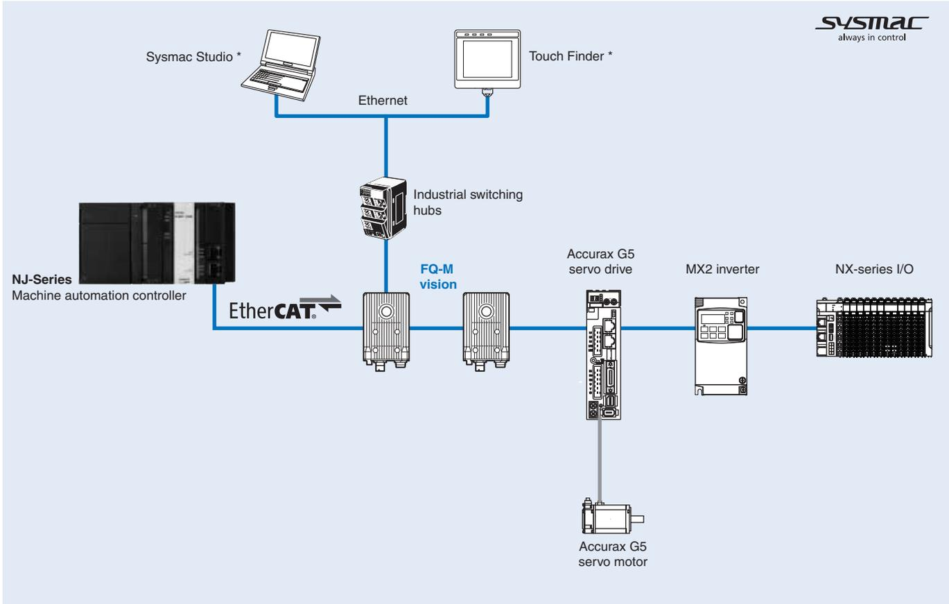
\* Sysmac Studio and Touch Finder can not be used together. When both are connected, Sysmac Studio will have a priority. When you use the Sysmac Studio Standard Edition and connect the FQ-M Series and the Machine Automation Controller NJ-Series, connect them with a general-purpose Ethernet cable or a USB cable.
