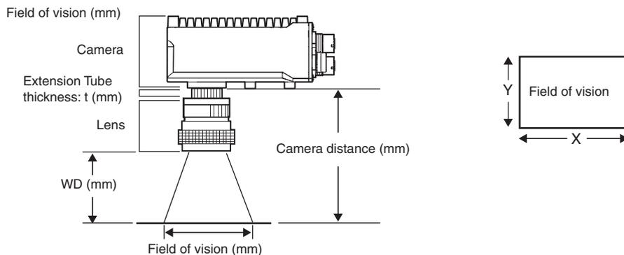
\*1. The lengths of the fields of vision given in the optical charts are the lengths of the Y axis.
