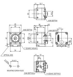
\* The base at the bottom of the camera can be mounted to the bottom, top, and both sides. Remove the base mounting screw (M4x8) and correct the mounting position. (Recommended mounting screw torque: 1.2 N·m)
