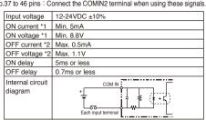
\*1 ON current/voltage means the current or voltage value to activate the terminal. The ON voltage value is the potential difference between COM IN and each input terminal.
