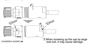
· When a gap between a mold cover of contact block and a cap disappeared assembly and wire connection has completed.
