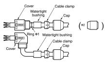
Insulation caps and insulation tubes are included with 5-pole Connectors (XS $\square$ C-D5S $\square$  and XS $\square$ G-D5S $\square$ ).
