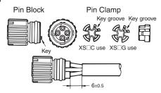
Tentatively insert the pins to the pin block holes so that the key on the pin block will coincide with the key groove on the pin clamp.
