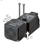
When positioning the sensing surface to the side, rotate it to the required position, then fit it into the case. (The possible positions are 0, 90, 180, and 270°. Do not forcefully rotate the sensing surface.)
