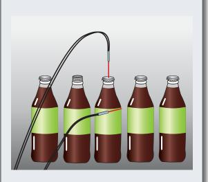
One sensor head detects the bottle's leading edge while the other inspects for cap presence. If both outputs are ON, the cap is in place.
