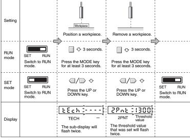
If the output setting is set to 1-2 (differential operation), the value between the two differential values when teaching is performed is used as the threshold setting.
