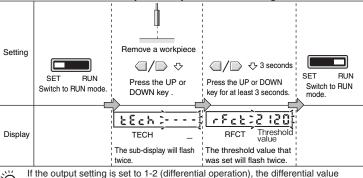
If the output setting is set to 1-2 (differential operation), the differential value when teaching is performed is used as the threshold setting for channel 2. (Same as for Teaching for Through-beam Sensor Heads.)
