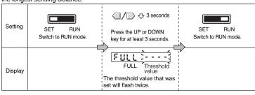
It does not matter whether or not there is a workpiece. The value that is set will depend on the detection method and power adjustment
