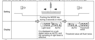
If the output setting is set to 1-2 (differential operation), the value between the detected maximum and the minimum differential values when teaching is performed is used as the threshold setting.
