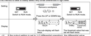
when teaching is performed is used as the threshold setting for channel 2. (Same as for Teaching for Reflective Sensor Heads.)
