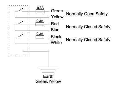
NOTE: Contacts shown when the actuator is in place.
