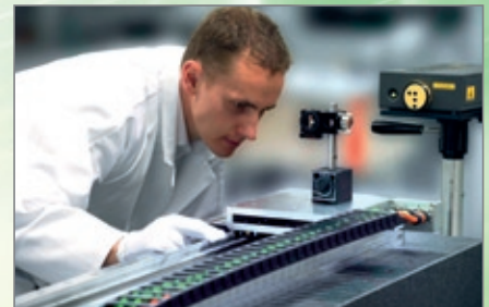
Precision measurement with laser interferometer for quality assurance to create the data for stage mapping.
