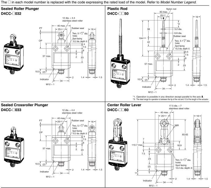
Note: Unless otherwise specified, a tolerance of  $\pm 0.4$  mm applies to all dimensions.
